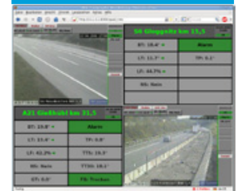
BT: Ground temperature LT: Air temperature LF: Air humidity NS: Precipitation
